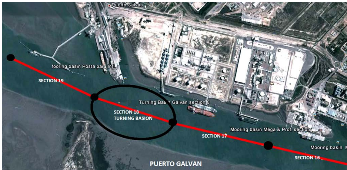
Figure 11: Sections and turning basins Puerto Galvan
